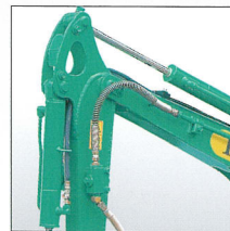
Auxiliary Hydraulic Piping
